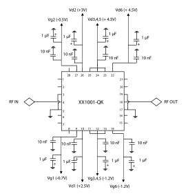
**App Note [1] Biasing** - Please refer to the application diagram above for recommended biasing information. The table below shows the recommended drain currents for each stage.
